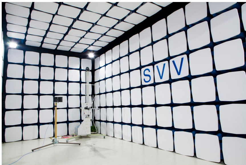
Image of SVV's EMC chamber in Shenzhen, China, for testing connected devices
